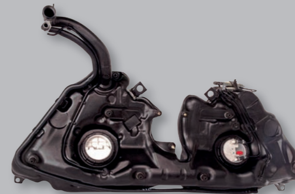
Multi-layer plastic fuel tank for the Mercedes Type W202 (C-Class from 1993)
