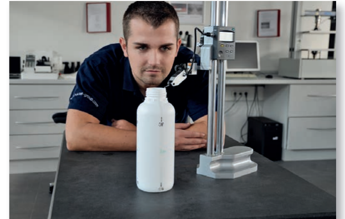
Technikum employee measuring a HDPE bottle
