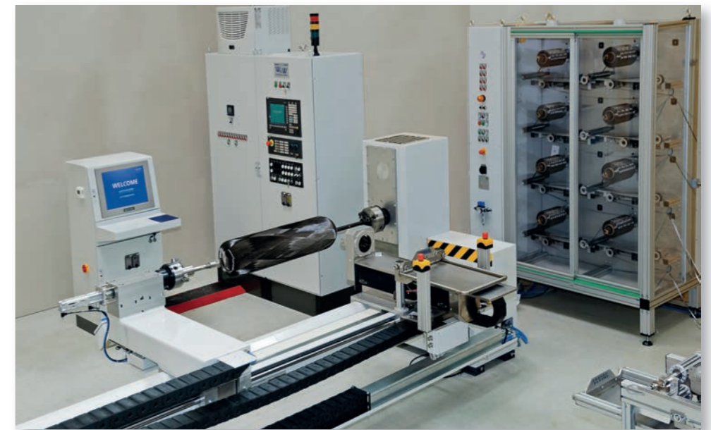
Production system for composite vessels in the Technikum (detail)
