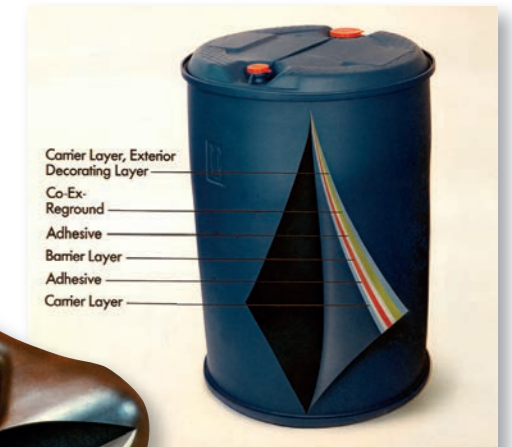
Schematic diagram of the six layers of the coextrusion, using a tank as an example
