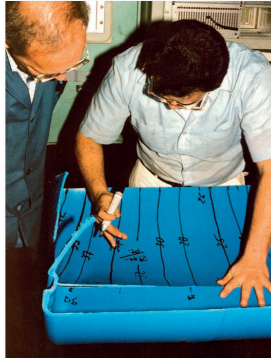
Checking the wall thickness distribution on the Super Handling tank
