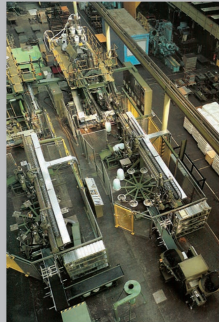
Production line for fully automated production and quality control of 30 liter canisters and 120/220 liter drums, 1990
