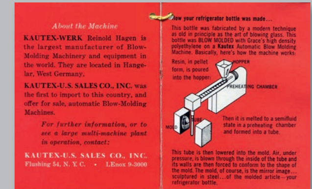
Product insert for the American department store chain, Macy's, shows customers how their plastic bottle was manufactured.
